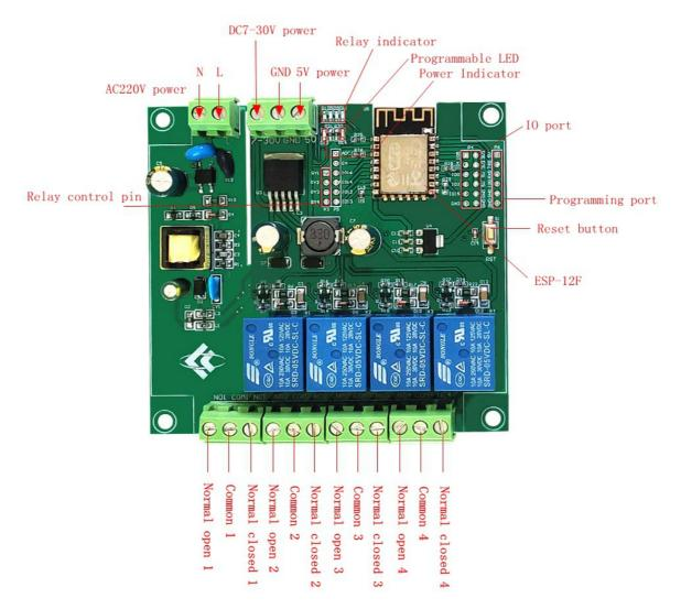
Programming port: ESP8266's GND, RX, TX, 5V are respectively connected to the GND, TX, RX, 5V of the external TTL serial port module. IO0 needs to be connected to GND when downloading, and then disconnect the connection between IO0 and GND after the download is complete;
