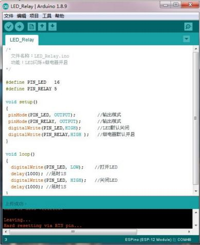
5. Finally, disconnect IO0 and GND, power on the development board again or press the reset button to run the program.
